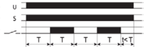
FZ32: Clock generator - Start after impulse
